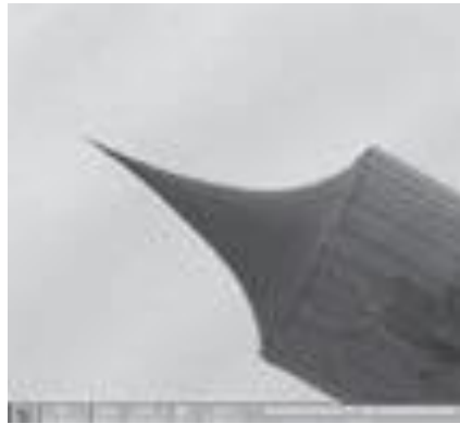
Figure 31: SEM image of a tungsten tip for STM imaging
